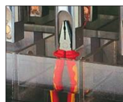
Dielectric water bath test to 10000 V.
