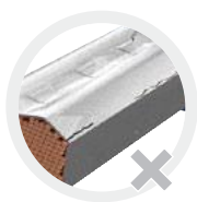
Formation of cracks at the impressions of the crimping jaw
