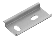
TS 35/7.5 mm according to EN 60715 (s = 1.0 mm)
