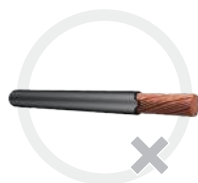
Insulation not cut in properly
