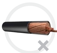
Pulled out conductor
