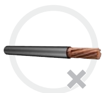
Damaged or cut-off individual wires
