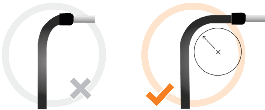
Risk of breakage due to overload
